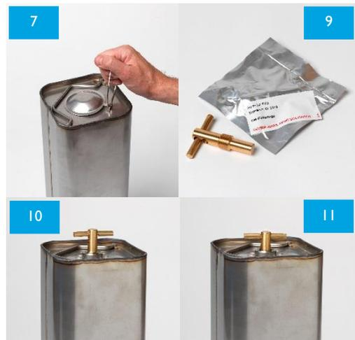
11. Screw the initiator fully into the top of the generator until it will go no further. The generator will start producing oxygen during this operation, although this may not be immediately apparent
