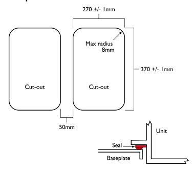
If the cartridges need to be secured in position the top edge of the base flange can be used to clamp against. Care should be exercised to ensure the base seal is not distorted to the point it fails to seal if the cartridges are fastened or clamped in position. The outside edge of the upper surface can be used to seal against if the cartridges are to be used in a fully ducted system.
