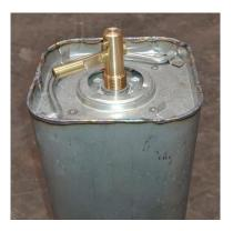
12. After approximately 90 minutes the oxygen flow will stop, but the unit will remain very hot for some considerable time. AVOID CONTACT WITH HOT UNITS
