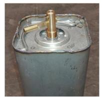
12. After approximately 90 minutes the oxygen flow will stop, but the unit will remain very hot for some considerable time. AVOID CONTACT WITH HOT UNITS
