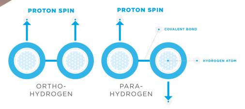
Fast catalysis during liquefaction ensures that only para hydrogen is present for storage. This results in less than 1% percent hydrogen loss per day in a well-insulated Dewar, compared to 18% per day without lonex<sup>®</sup> Type OP Catalyst.
